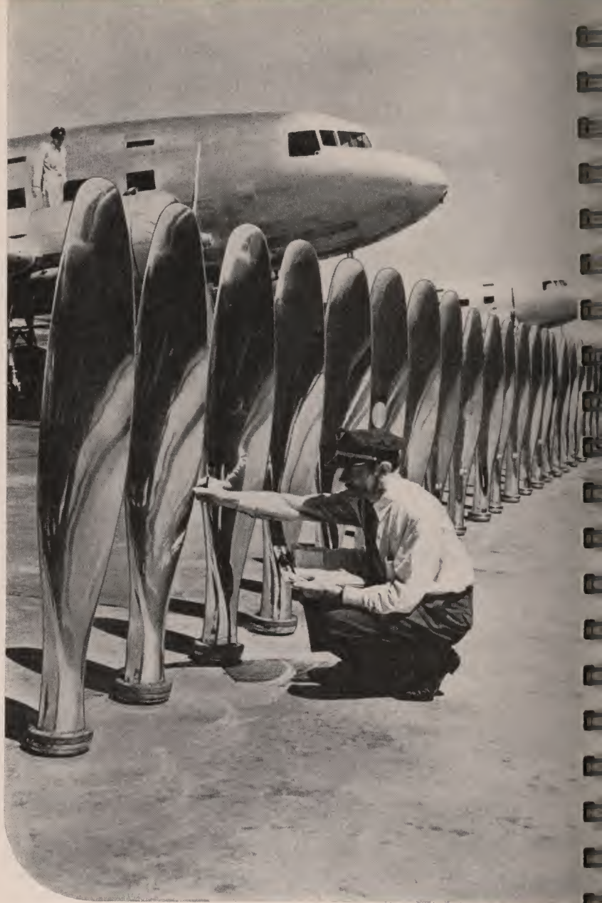
Forged aluminum alloy propeller blades.
